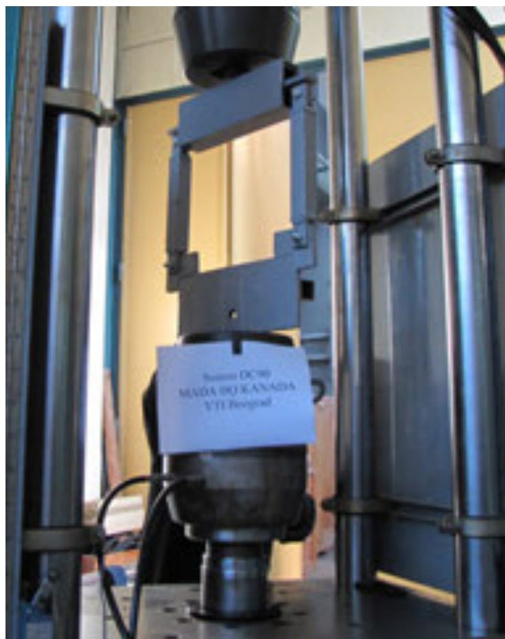
Figure 3 Test set-up of MADA HQ Kanada damper
