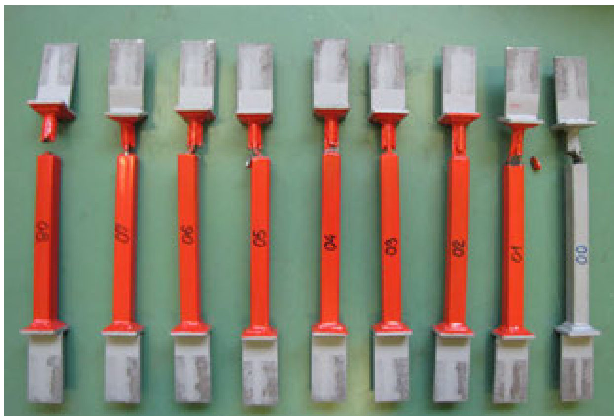
Pic. 35. View of broken samples after the testing
