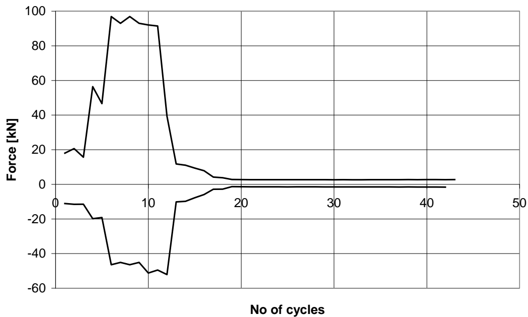
Figure 18 Maximum/minimum force vs. number of cycles
