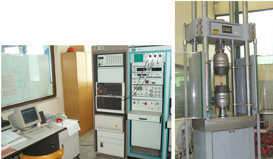
Figure 2. MTS Servo-controlled Hydraulic System
