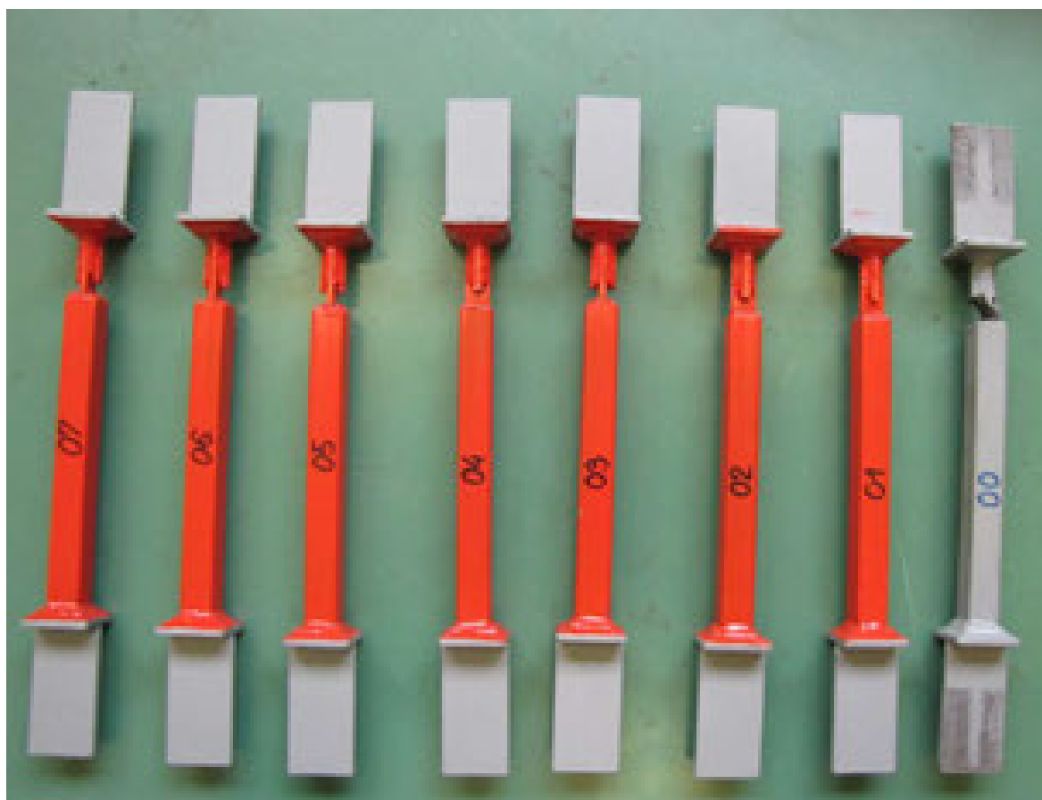
Picture 1 Dampers – absorbers of seismic energy HQM
