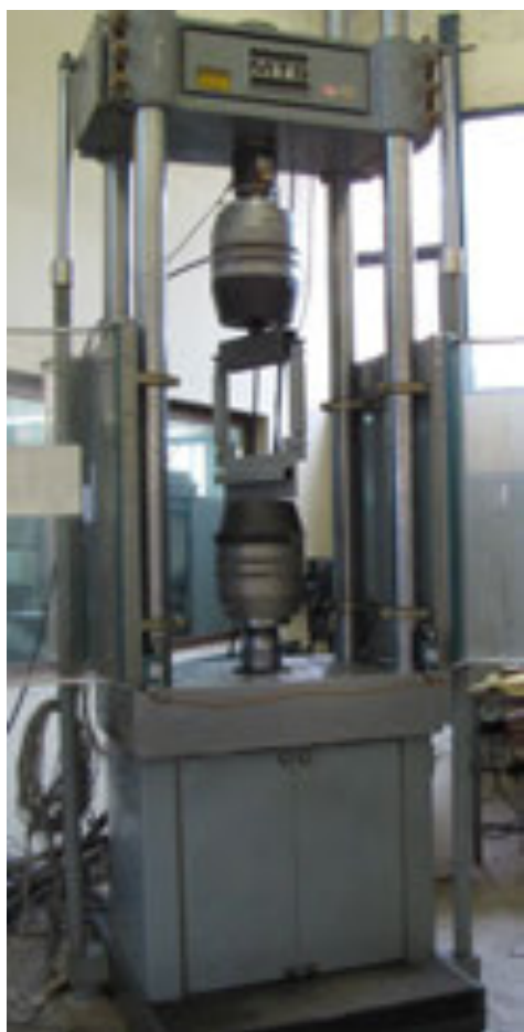
Figure 3 Test set-up of MADA HQ Kanada damper
