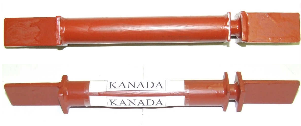
Figure 1. View of Damper type “Canada” (absorber of seismic energy).
