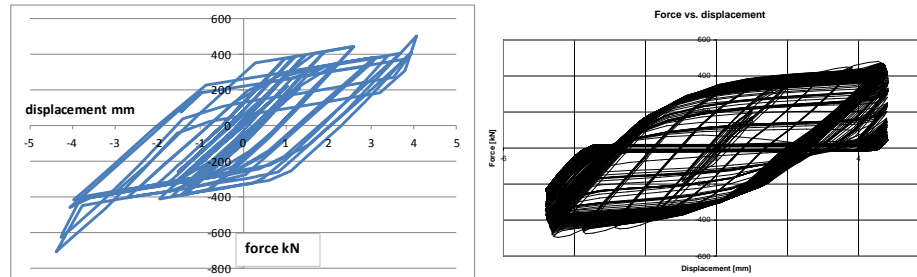
Figure 6. (a) D-98 Damper 1.5 to 4.0 mm , F=320-400 kN (b) Damper 1.5 to 4.5 mm; 450 kN (test) Hysteresis obtained from the analysis (a); Results from the test (b)
