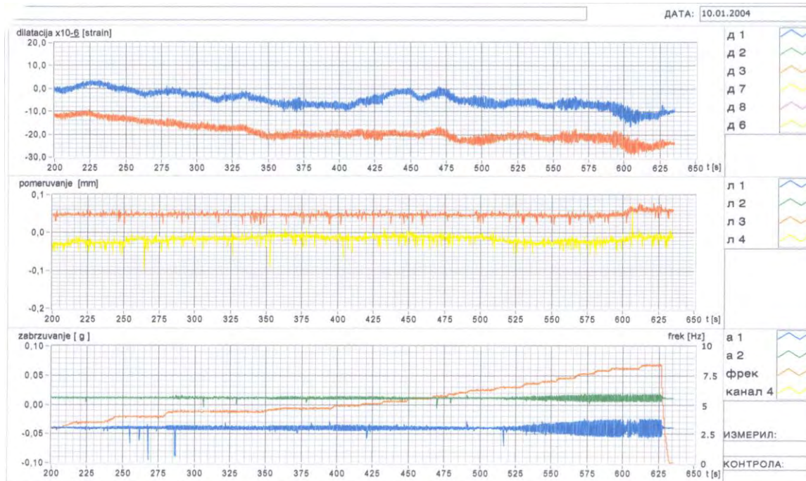
Fig.15. Time history records of strain, displacement and acceleration at characteristic points; Test 5, Disposition 2, Longitudinal direction
