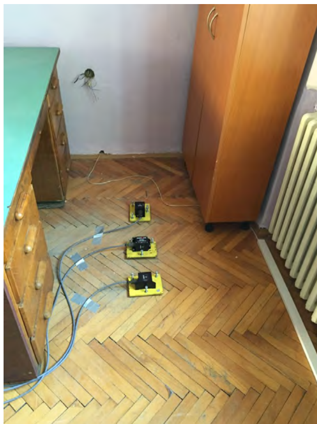
Fig. 2-4 Location of the uni-axial reference sensors in point F on the 2 nd floor.
