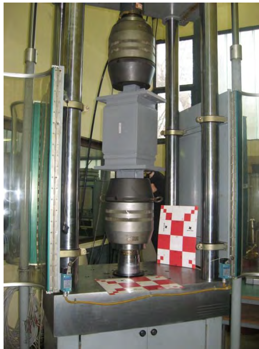
Figure 1. AFS, Servo-controlled Hydraulic System
