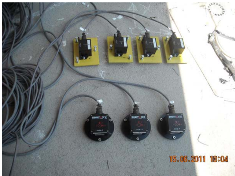
Figure 12. Dynamic calibration test of DIGITEXX accelerometers
