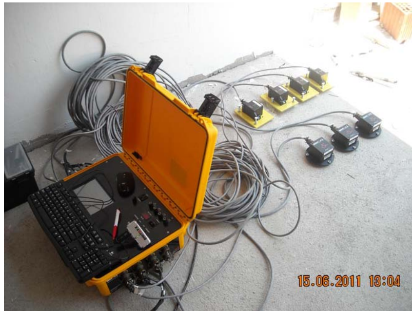
Figure 10. DIGITEXX PDAQ 16 channels data acquisition system and accelerometers type D110-T and D110-U used for ambient vibration measurements
