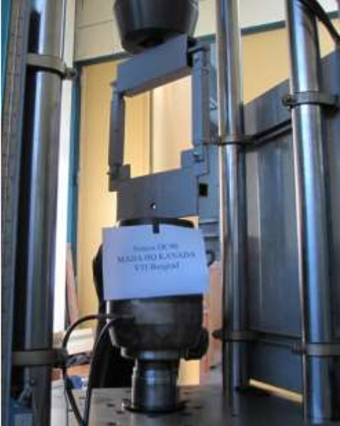
Test set-up of MADA HQ Kanada damper The first specimen complete hysteresis (force s. displacement)
