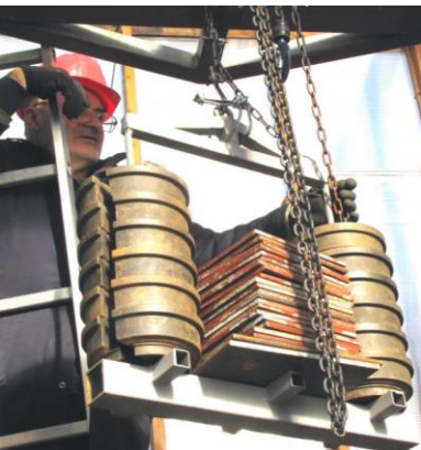
Suspension and load introduction into the 118 CRANE TRACK
