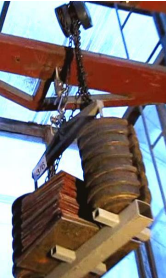
Suspension and load introduction into the 046 ADAPTER
