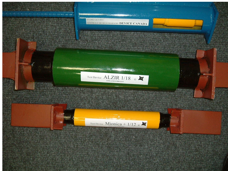
Figure 8. Typical dampers of DC 90 system
