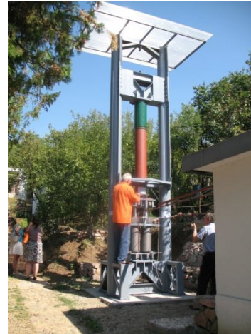
Figure 3. Damper Tipe "Vogzal" in the frame for testing
