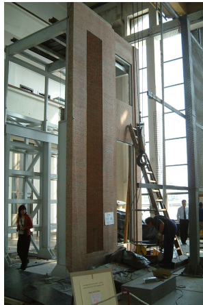
Figure 5 . Model of the wall of hydro-generator "Beauharnois" in 1:3 ratio on vybro-platform
