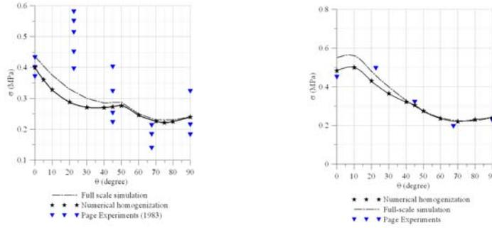
**Figure 3.** The distribution pattern Directional strength characteristic for uniaxial tension and biaxial compression-tension; comparison between the results for the full-scale and REV simulations
