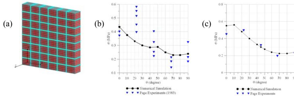
**Figure 1.** Numerical simulations of panels tested by Page (1983); (a) FE discretization; (b) & (c) failure envelopes for uniaxial tension and biaxial compression-tension ( $\sigma_c/\sigma_t=1.0$ ), respectively
