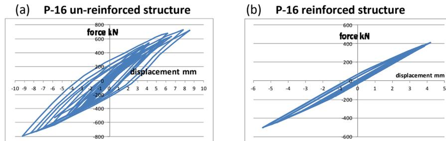
**Figure 9.** Hysteresis for a typical masonry panel obtained from the analysis: (a) before and (b) after the structural reinforcement with bracings and dampers
