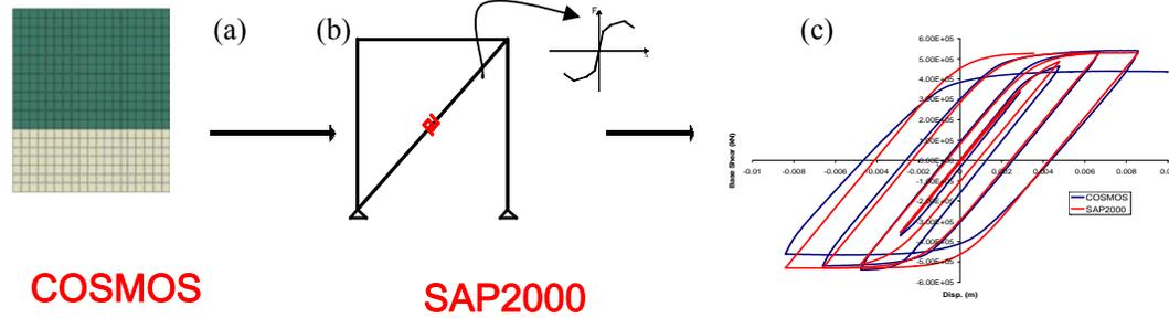
**Figure 6.** Typical masonry panel (a); replaced by “Link” element (b); having equivalent hysteresis (c)
