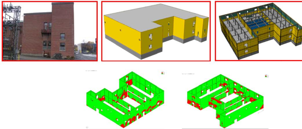
**Figure 4.** The geometry of the building, and the results of the elaborate FE dynamic analysis. The red areas indicate distribution of cracks in the masonry walls.
