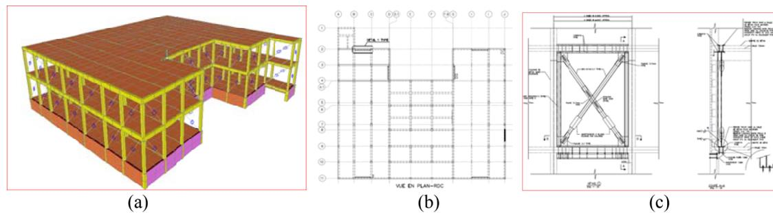
**Figure 7.** Numerical model including the “Link” elements in SAP2000 (a); location of the bracings with dampers on the ground floor of the building (b); and unit of bracing with dampers (c)
