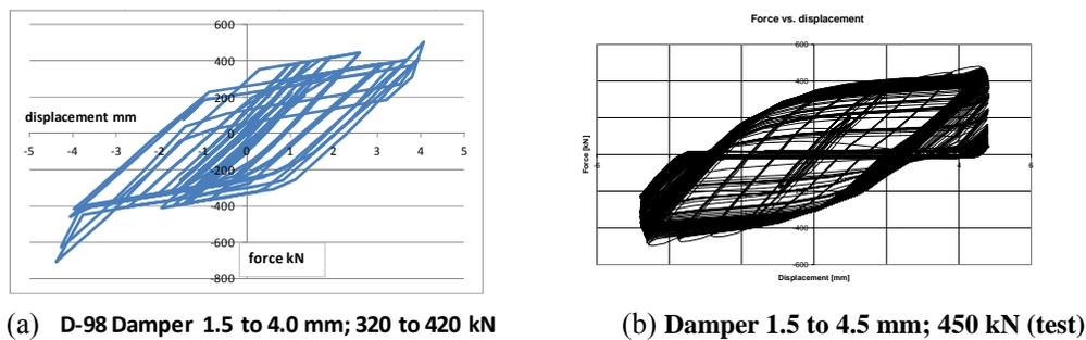
**Figure 8.** Hysteresis obtained from the analysis (a); Results from the test (b)
