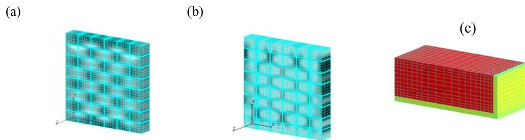
**Figure 2.** The distribution pattern of (a) maximum principal stress; (b) minimum principal stress in biaxial tension-compression  $\theta=10^\circ$ ; (c) REV and its finite element discretization
