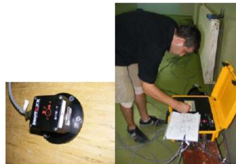
Digitex accelerometer high sensitivity and accuracy of +- 0.1% and a system for acquisition and signal conversion
